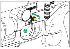
To secure the gun push the safety (A) from the left side of the gun body. Moving the button locks the weapon. At this point the weapon is secured against fire.
