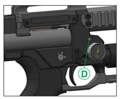
Tighten in the bleed screw (D) and refill the rifle with air (you may need to cock the rifle during this step).
